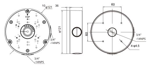
There are three pipe thread interface in the junction box, one of which needs to be used, so our company provides two plugs.
