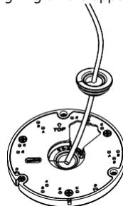
3. Plug the silicon plug into the upper cover, connect the upper cover and base, then attach camera to the upper cover plate. Pay attention to select correct screw holes to match the different model type.
